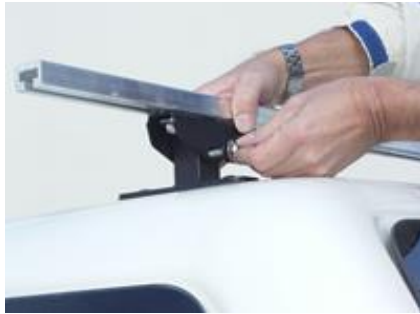
INSERT SCREW CONNECTING FOOT TO CROSSBAR...
