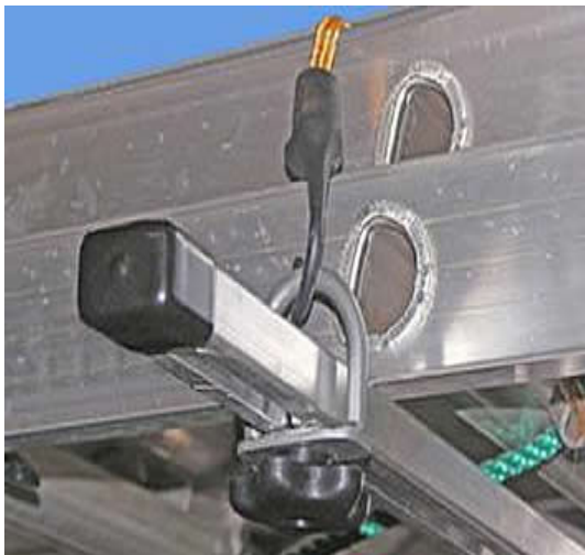
USING THE ADJUSTABLE TIE-DOWNS TO TIE-DOWN LADDERS OR OTHER CARGO IS EASY
