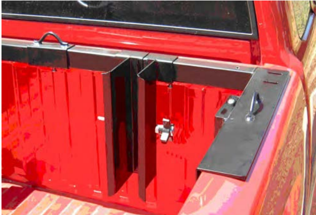
Fig 7. Grip Chock before adjustment
