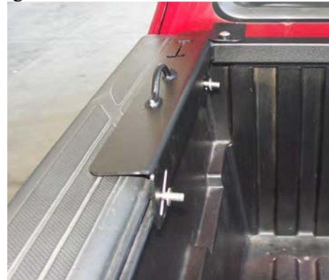
Fig. 17 Slide slots over inserts add washers
