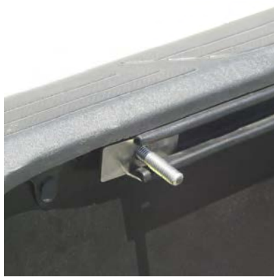
Fig. 14 Slide insert into track
