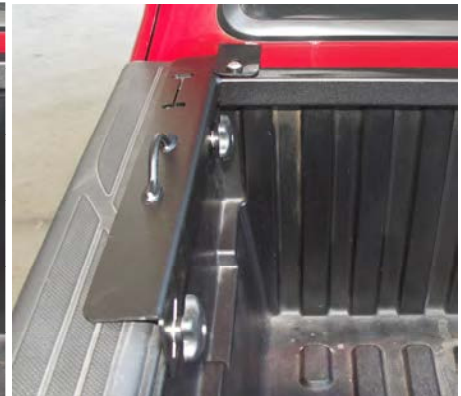
Fig. 18 Tighten knobs on inserts
