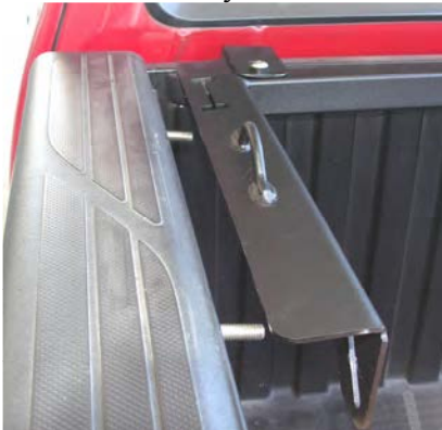
Fig. 16 Align inserts with slots
