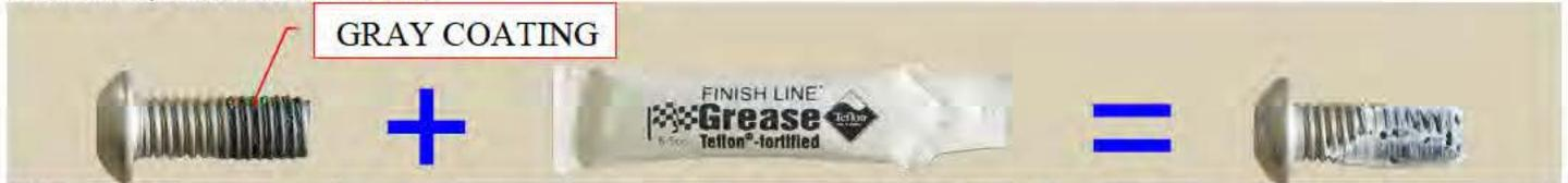
**IMPORTANT:** ALL Stainless Steel Screws have been DIPPED IN A GRAY COATING to help prevent threaded parts from sticking together. However, you should have also received a small tube of grease. Coat the threads of ALL SCREWS with grease BEFORE ASSEMBLY TO MAKE ASSEMBLY EASIER AND TO PREVENT THEM FROM SEIZING-UP DURING DISASSEMBLY.
