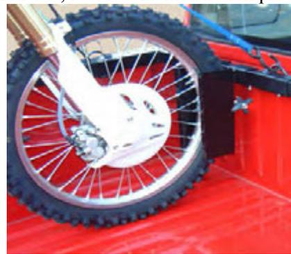
Fig 22. Motorcycle Rack with Grip Chocks
