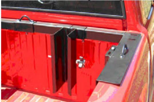
Fig. 7. Grip Chock before adjustment
