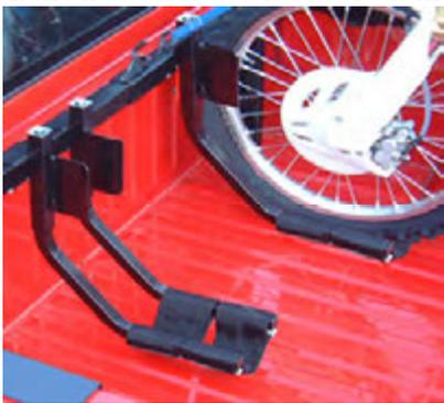
Fig 21. Motorcycle Rack with Cradle Chocks
