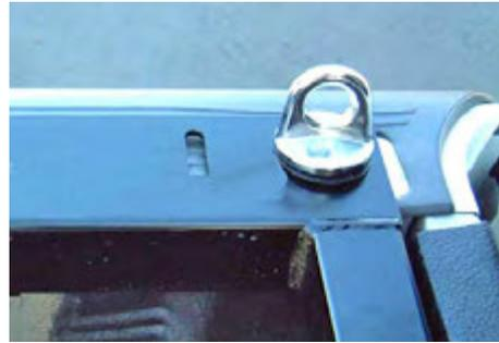
Fig 20. Islet screwed into stake pocket
