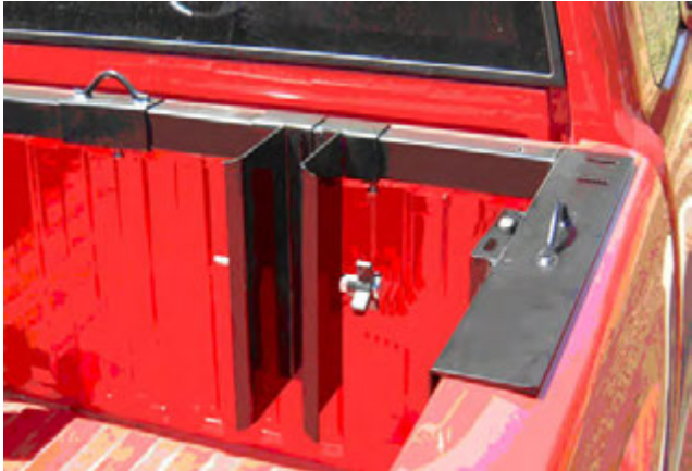
Figs 7. Grip Chock before adjustment
