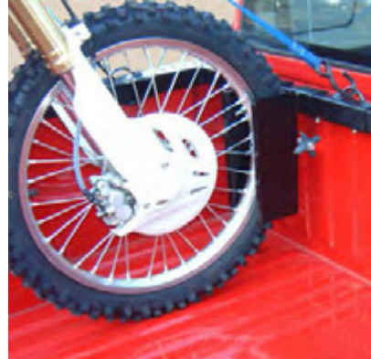
Fig. 12 Grip Chock installed
