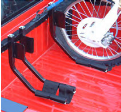
Fig. 19 Cradle Chocks installed
