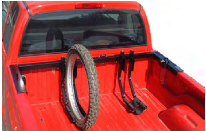
Figs 4. & 5. Wheel chock and receiver during assembly Fig 6. Mounted rack with wheel in webbing of wheel chock
