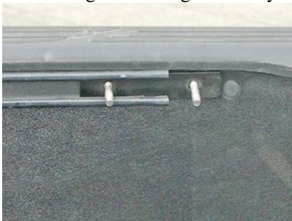
FIG. B – Push Insert into Track
