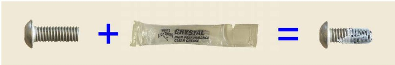
**A SMALL PACKET OF GREASE SHOULD BE INCLUDED IN YOUR PACKAGE. PLACE A DAB OF GREASE ON EACH SCREW TO MAKE THREADING EASIER AND HELP PREVENT SEIZING.**
