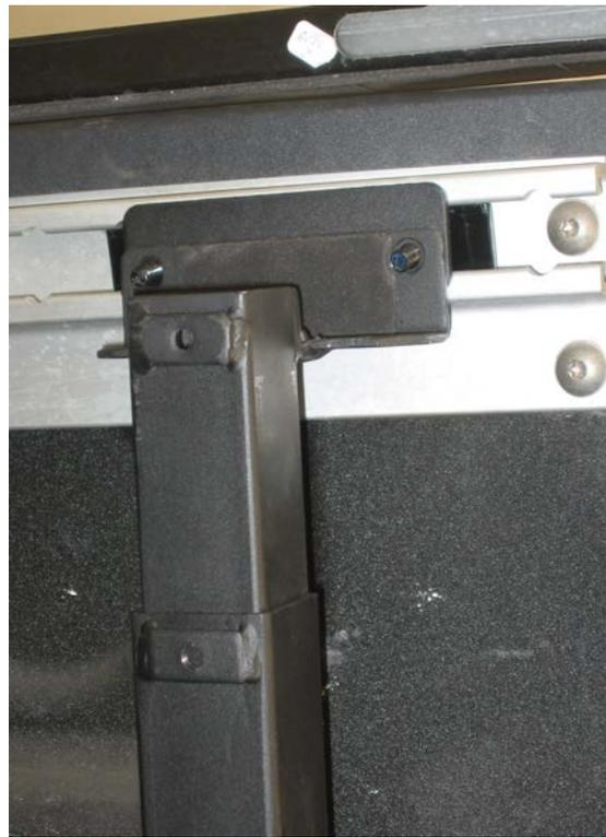
FIG. G – Alternate orientation for Base of Rack      FIG. H – During installation on Nissan Utili-track
