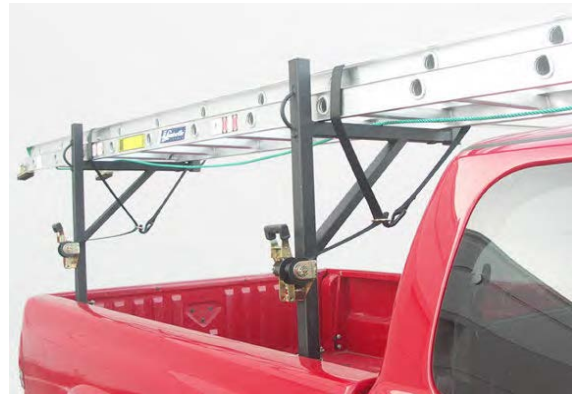
FIG 13 STEP 2 – Drape Ladder and Hook Strap
