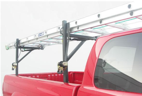
FIG 14 STEP 3 – Tighten Ratchet
