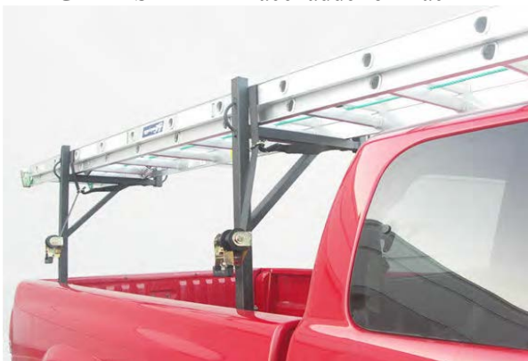
FIG 14 STEP 3 – Tighten Ratchet
