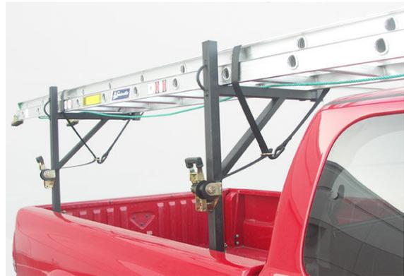
FIG 13 STEP 2 – Drape Ladder and Hook Strap
