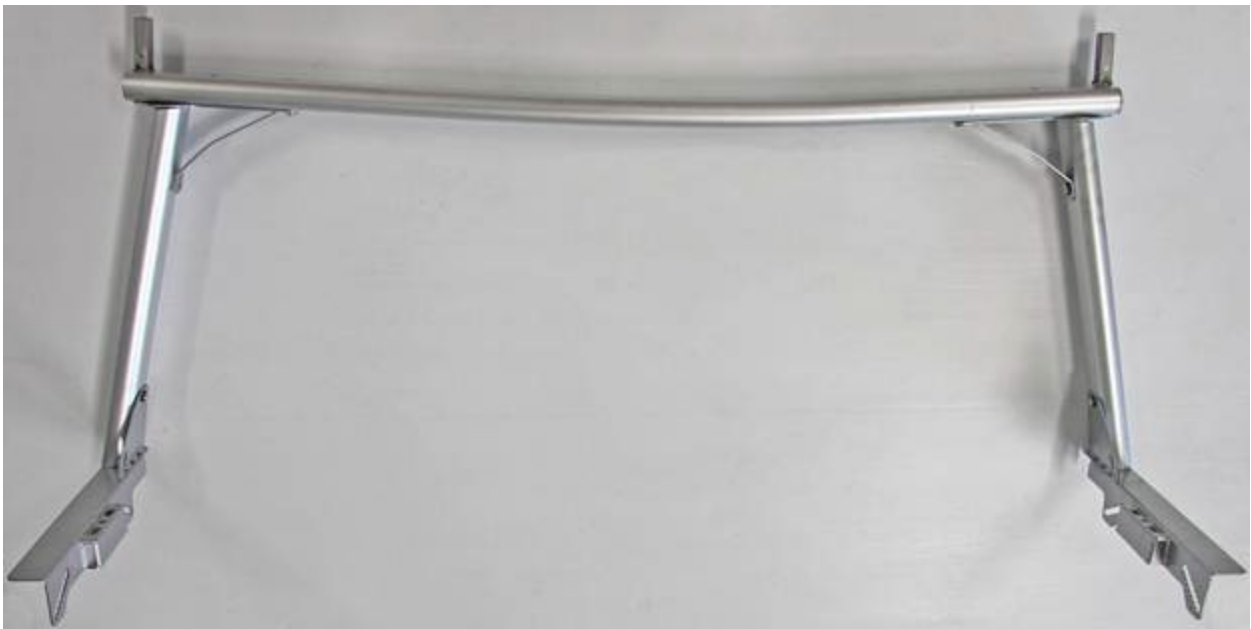
BENT WINDSTREAMER RACK SHOWN AFTER THE TEST AT OVER 1,890 lbs.
