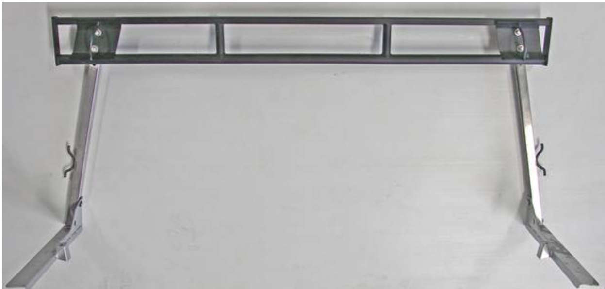
SLIGHTLY BENT DUAL RACK SHOWN AFTER THE TEST AT OVER 1,000 lbs.
