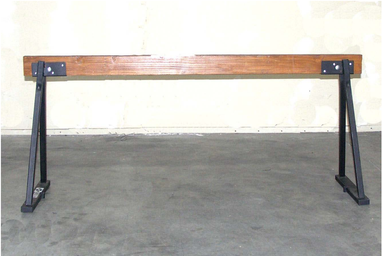
SAWHORSE RACK SHOWN AFTER TEST AT OVER 3,000 LBS.
