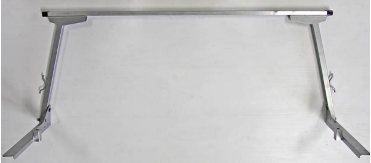
SLIGHTLY BENT PADDLER'S RACK SHOWN AFTER THE TEST AT OVER 900 lbs.
