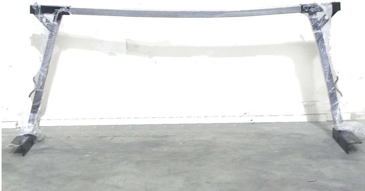
OLDER STYLE RAIL RACK SHOWN AFTER TEST AT OVER 2,700 LBS.
