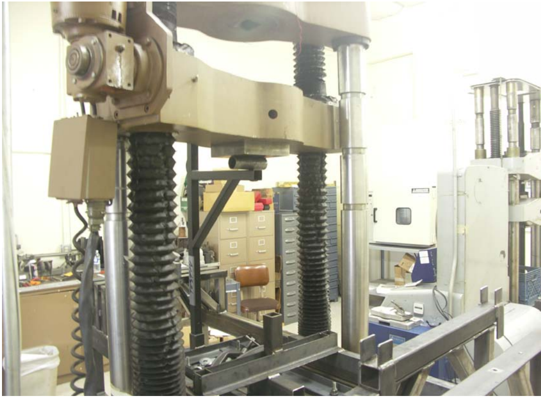
TEST APPARATUS WITH STRONG-ENDER LADDER RACK DURING TEST
