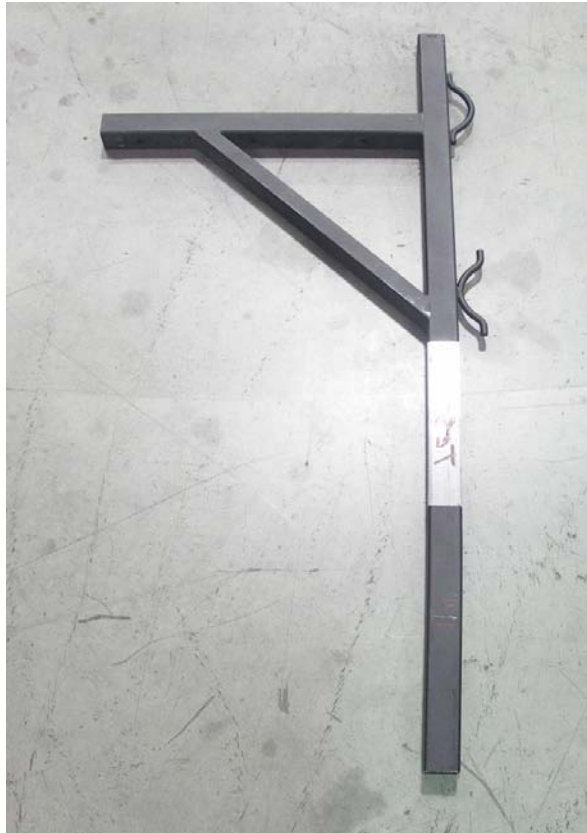
BENT STRUCTURAL FRAME of THE STRONG-ENDER RACK SHOWN AFTER TEST AT OVER 610 LBS.
