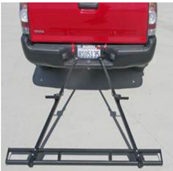
V-Rack lets you lower tailgate with rack attached or lower rack to the ground before opening the tailgate
