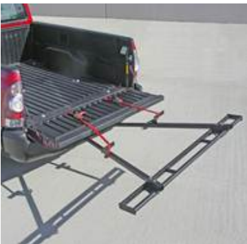
V-Rack lets you lower tailgate with rack attached or lower rack to the ground before opening the tailgate
